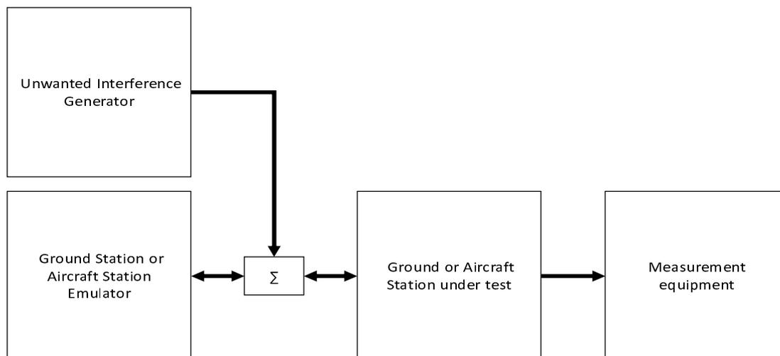
The insertion loss of the combiner shall be calibrated and taken into account when making measurements.
