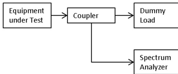
**Figure 3: Measurement Arrangement for Spurious emissions of transmitter measurement**
