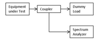
Figure 2: Test setup for residual power output test
