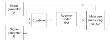
Figure 6: Arrangement for blocking measurement
