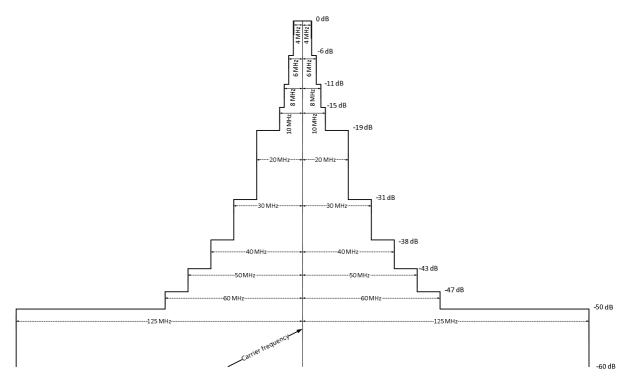
Figure 1: Spectrum mask for an interrogator transmitter
