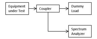
Figure 7: Measurement arrangement for receiver spurious emissions measurement
