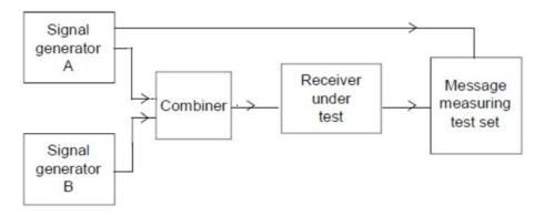
Figure 5: Measurement arrangement for co-channel rejection measurement
