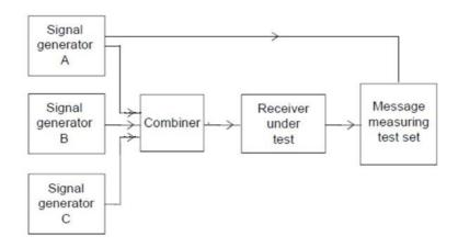
Figure 4: Measurement arrangement
