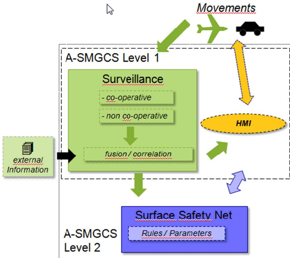
**Figure 1: A-SMGCS Level 1 and 2 Functional Configuration**
