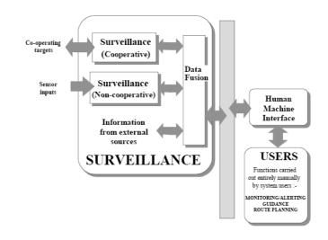
Figure 1: A-SMGCS Level 1 Functional Configuration
