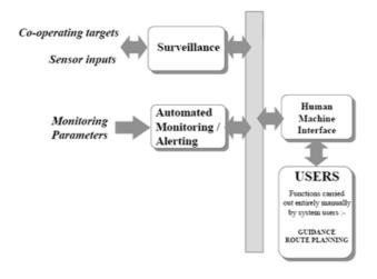
Figure 2: A-SMGCS Level 2 Functional Configuration
