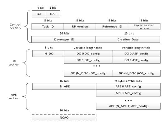
Figure 7.2: Binary format for Configcodes
