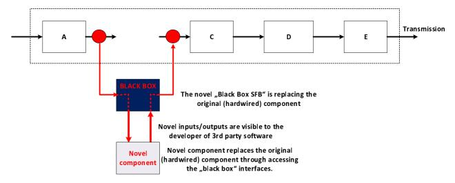
Figure C.2: Example replacement of a component through interfacing with novel SFB provided by a (3<sup>rd</sup> party) software provider
