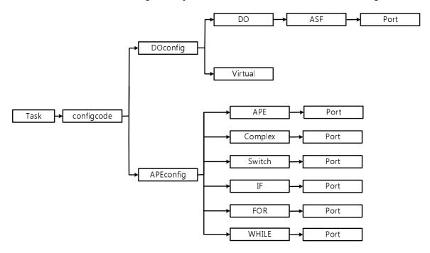
Figure 7.8: XML elements consisting of Configcodes
