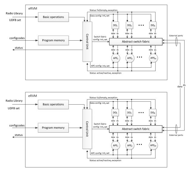
Figure 6.7: Horizontal scaling of eRVM
