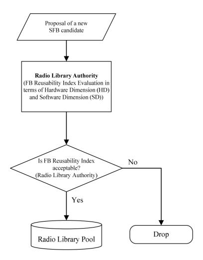
Figure D.1: Flow chart for determining SFBs
