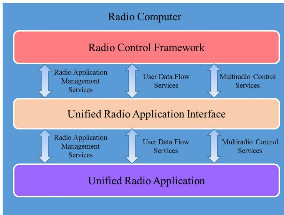
**Figure 5.1: Interconnection between RCF and URA using URAI for Reconfigurable MD**
