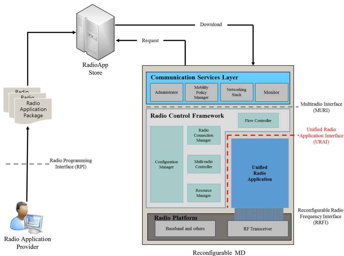
**Figure 4.1: Four sets of interfaces for Reconfigurable MD**
