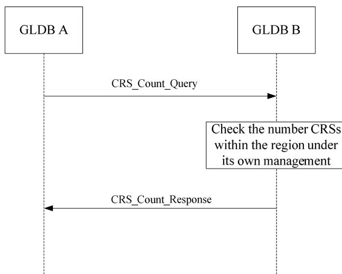
**Figure 6.8: CRS number discovery procedure**
