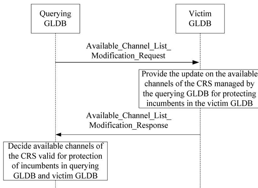
**Figure 6.5: CRS spectrum usage modification procedure (variant 2)**
