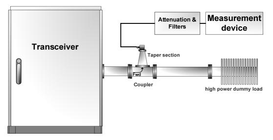
Figure B.1: Indirect method for radio frequency measurements with dismounted antenna
