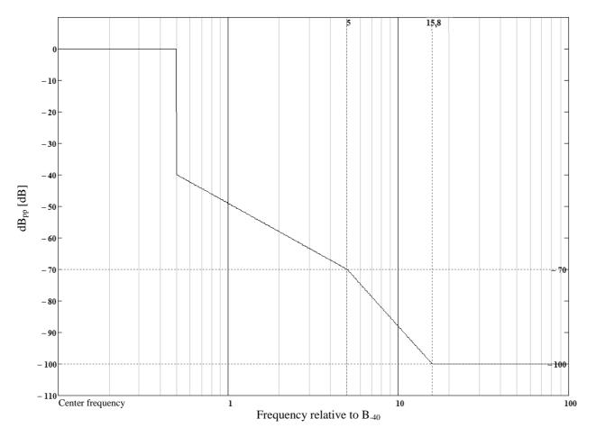
Figure 2: Out-of-Band emission limit masks
