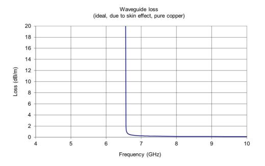
Figure E.1: Attenuation for an ideal waveguide
