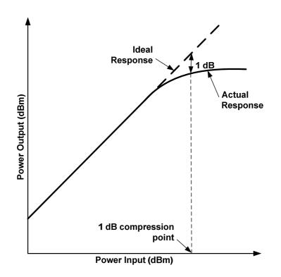
Figure 4: Receiver 1 dB compression point
