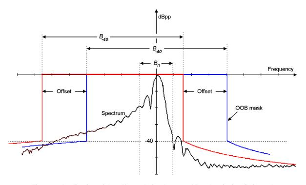
Figure 1: Application of the offset-rule for the Out-of-Band emission limit mask
