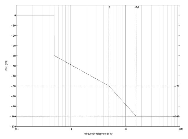
Figure 2: Out-of-Band emission limit masks
