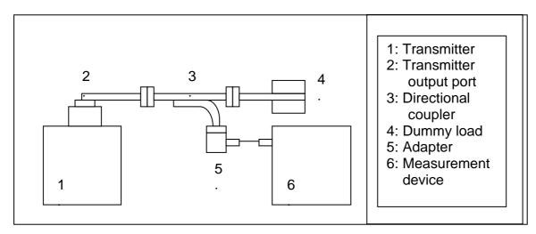
Figure B.1: Indirect method for radio frequency measurements with dismounted antenna
