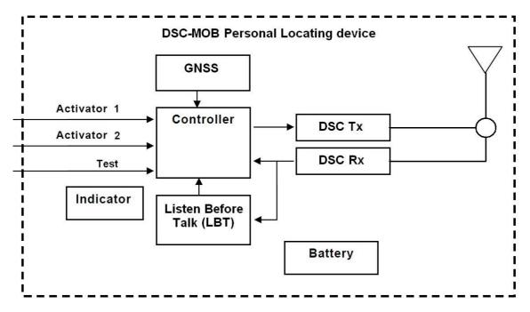
Figure 1: Functional block diagram of personal locating beacon
