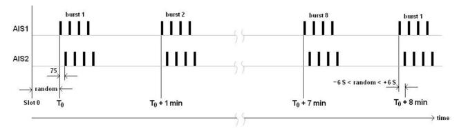
Figure 2: Burst transmissions in active mode
