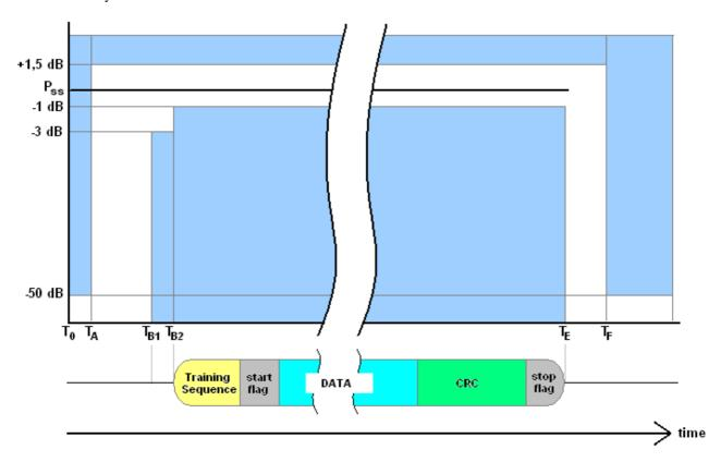
Figure 5: Power versus time mask
