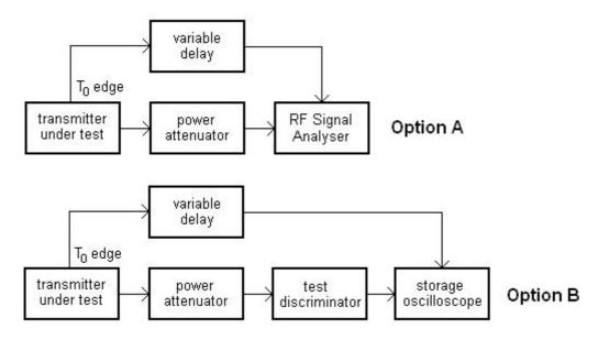
Figure 6: Measurement arrangement for modulation accuracy
