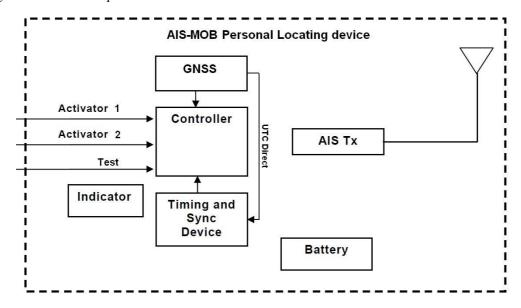
Figure 1: Functional block diagram of personal locating device
