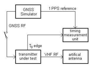
Figure 7: Measurement arrangement for synchronization accuracy
