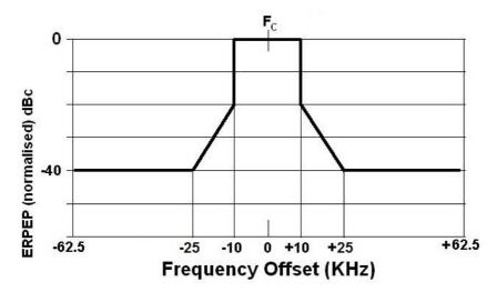
Figure 4: Transmitter spectrum mask
