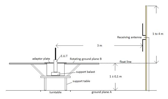
Figure C.1: Float-free test support
