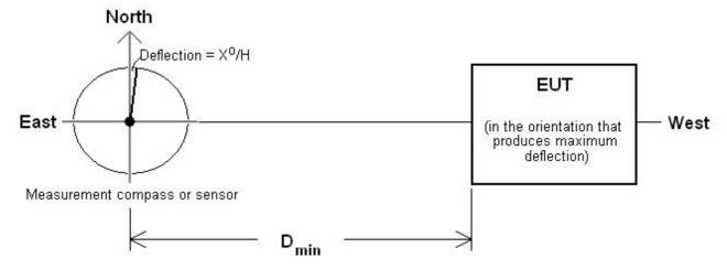
Figure 3: Compass safe distance test set up
