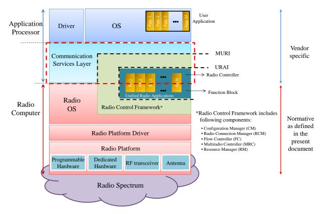
Figure 4.2: Reconfigurable Mobile Device (MD) architecture Reference Model for multiradio applications
