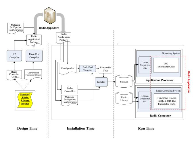
Figure 4.10: Conceptual Diagram of adopting platform-independent IR (dynamic linking) for radio application package for MDRC-5, MDRC-6 and MDRC-7
