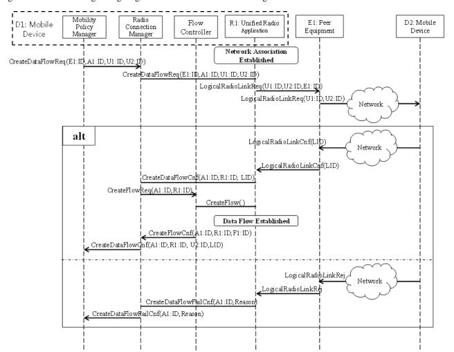
Figure 6.8 illustrates a signalling diagram related to the creation of a logical radio link association.
