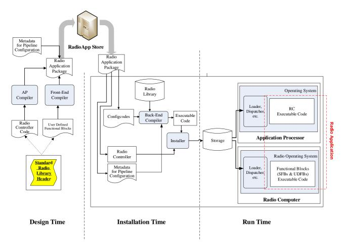
Figure 4.9: Conceptual Diagram of adopting platform-independent IR (static linking) for radio application package for MDRC-5, MDRC-6 and MDRC-7
