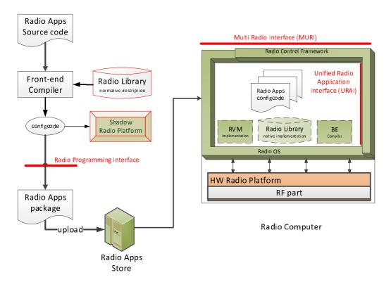
Figure 4.3: System architecture for Radio Computer where Radio Library and Back End (BE) compiler are included within the Radio Computer
