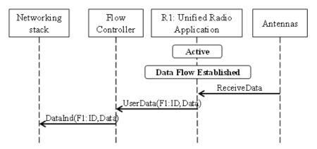
Figure 6.10: Signalling diagram of receiving data
