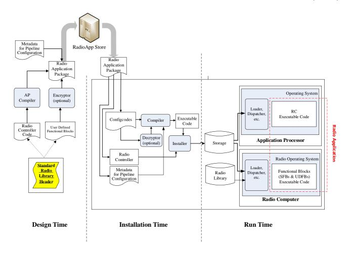
Figure 4.8: Conceptual Diagram of adopting platform-independent source code (dynamic linking) for radio application package for MDRC-5, MDRC-6 and MDRC-7
