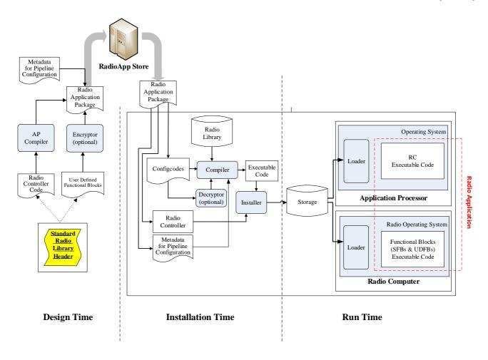
Figure 4.7: Conceptual Diagram of adopting platform-independent source code (static linking) for radio application package for MDRC-5, MDRC-6 and MDRC-7
