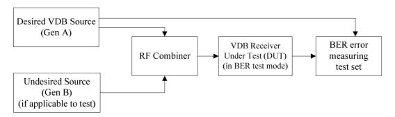
Figure 10: Receiver BER measurement
