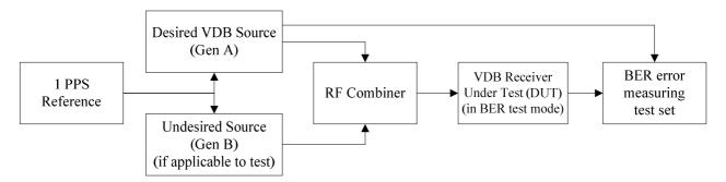
Figure 8: Time slot decoding measurement
