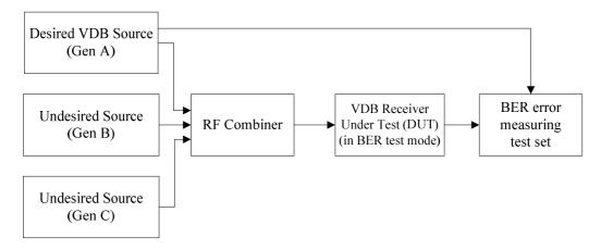
Figure 9: In band Intermodulation measurement
