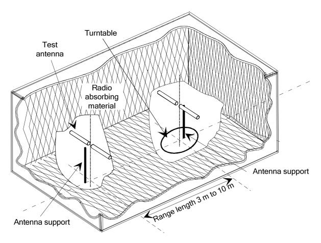
Figure B.1: A typical anechoic chamber
