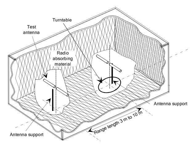
Figure B.1: A typical anechoic chamber
