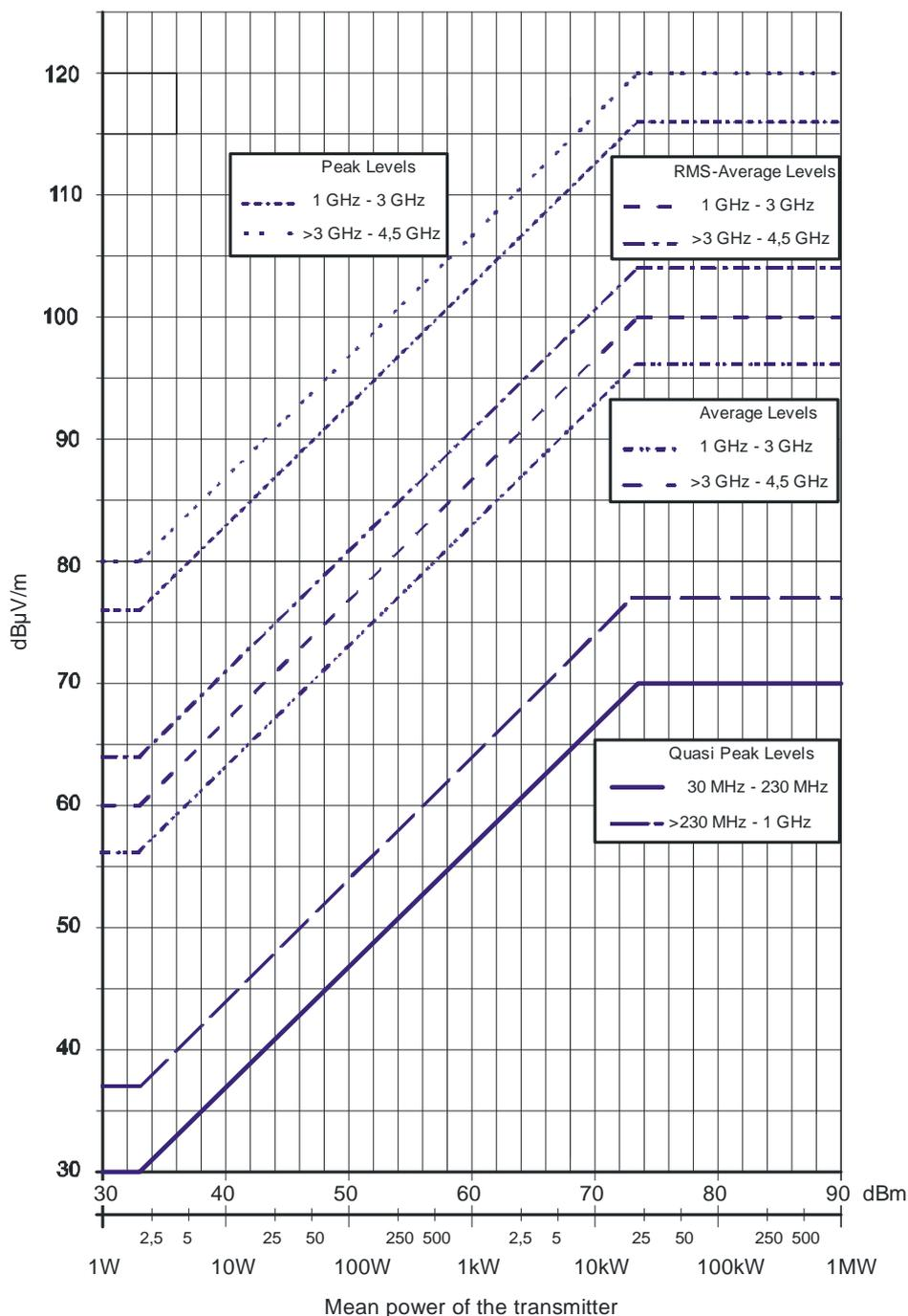
**Figure 4.5: Cabinet radiation limits for mobile TV transmitters 30 MHz to 4,5 GHz**
