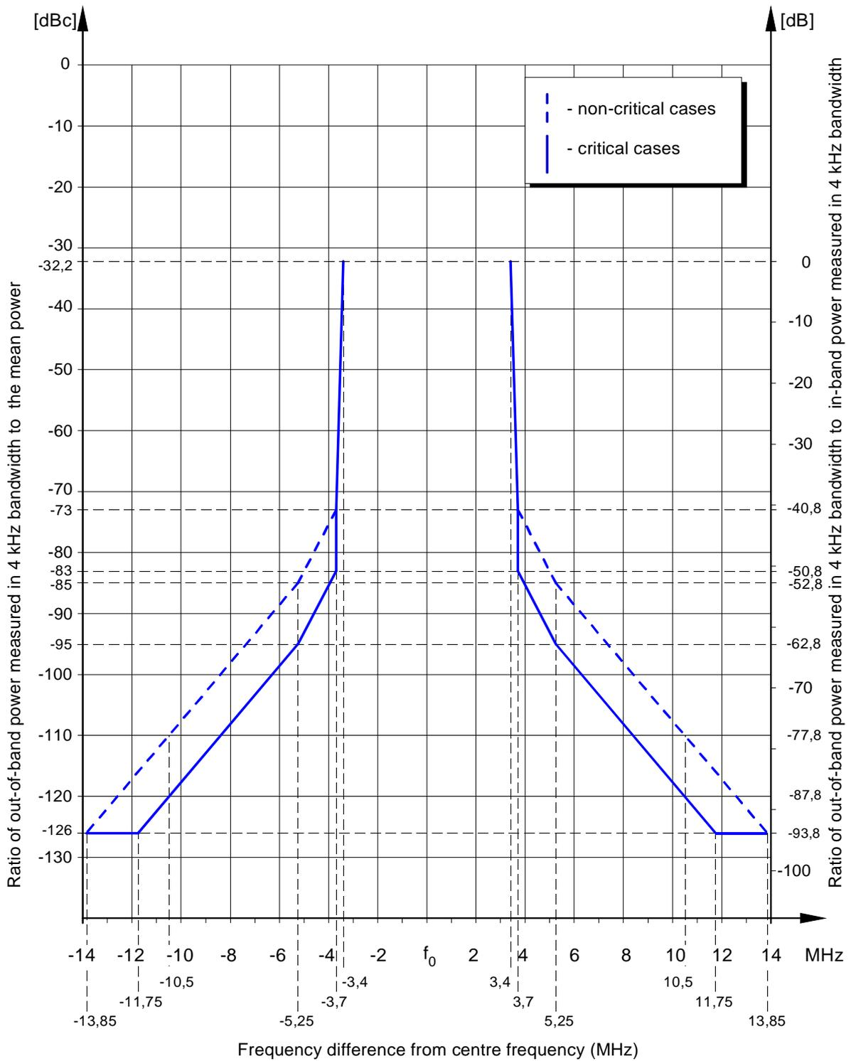
Figure 4.3: Out-of-band limits for mobile TV transmitters  $\geq 25$  W in 7 MHz channels
