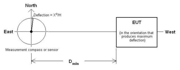
Figure 1: Compass safe distance test set up
