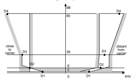
Figure B.1: IF filter characteristics
