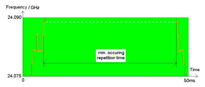
Figure 15: Example of a spectrogram for repetition time measurement
