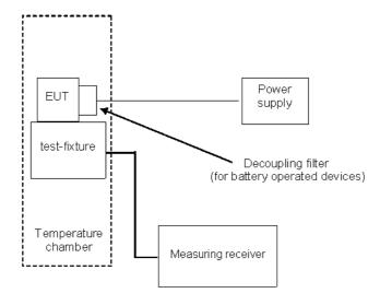
Figure 4: Measurement of EUT performance in temperature chamber
