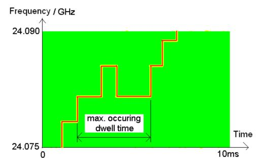
Figure 14: Example spectrogram of absolute dwell time measurement
