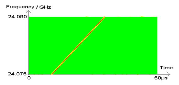
Figure 12: Example spectrogram of dwell time measurement
