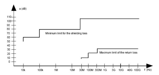
Figure A.3: Specification for shielding and reflections
