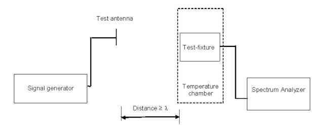
Figure 2: Validation of test fixture without EUT
