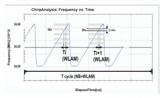
Figure B.3: Frequency versus Time of the WLAM Signal
