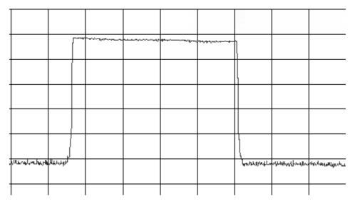
Figure B.2: Schematic example measurement of WLAM spectrum for determining the e.i.r.p. for sub-modes SM1, SM2 and SM3
