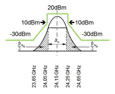
Figure 16: Out-of-band emissions (beta = 1, Bn = 200 MHz)
