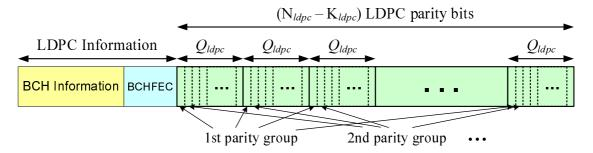
Figure 33: Parity bit groups in an FEC block
