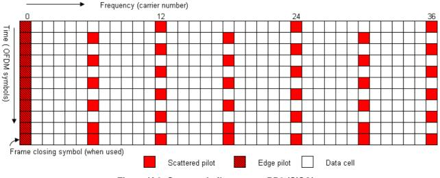
Figure K.2: Scattered pilot pattern PP2 (SISO)
