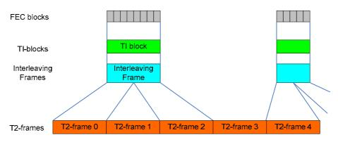
Figure 18(b): Time interleaving for  $P_{I}=2$ ,  $I_{JUMP}=2$ ,  $N_{TI}=1$
