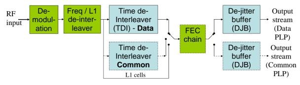
Figure C.2: Receiver buffer model
