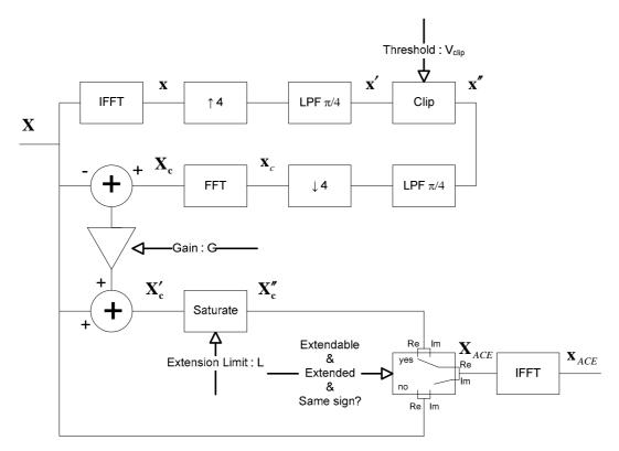
Figure 50: Implementation of the Active Constellation Extension algorithm
