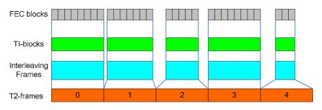
Figure 18(a): Time interleaving for  $P_{I}=1$ ,  $I_{JUMP}=1$ ,  $N_{TI}=1$
