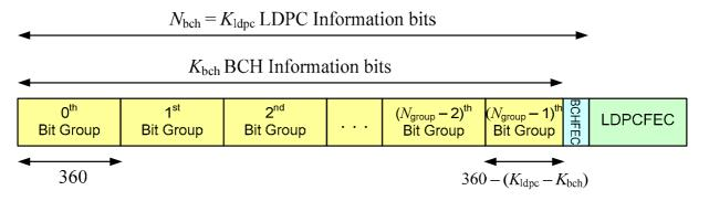
Figure 31: Format of data after LDPC encoding of L1 signalling
