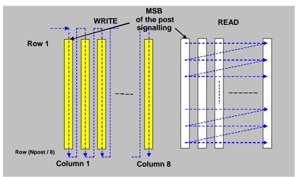
Figure 34: Bit Interleaving scheme for L1-post (16-QAM)
