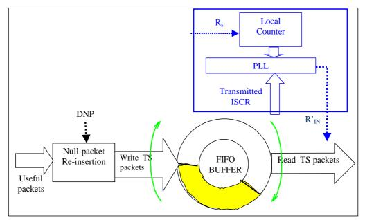
Figure J.1: Example receiver block diagram for Null-packet re-insertion and R<sub>TS</sub> clock recovery
