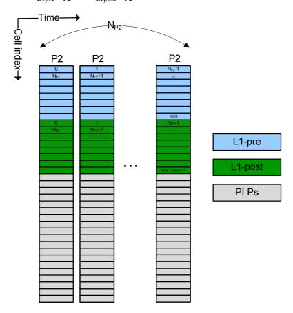
Figure 40: Mapping of L1 data into P2 symbol(s), showing the index of the cells within the L1-pre and L1-post data fields
