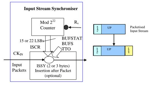
Figure C.1: Input stream synchronizer block diagram
