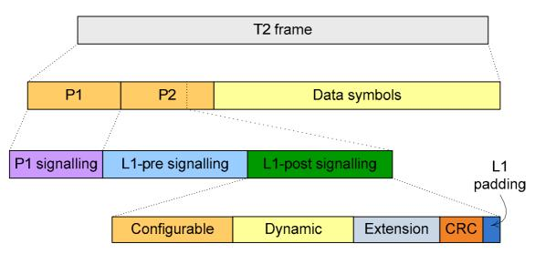
Figure 24: The L1 signalling structure
