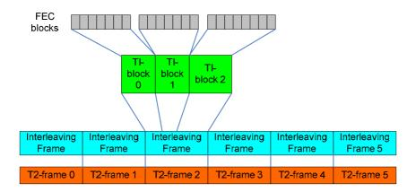
Figure 18(c): Time interleaving for P<sub>I</sub>=1, I<sub>JUMP</sub>=1, N<sub>TI</sub>=3
