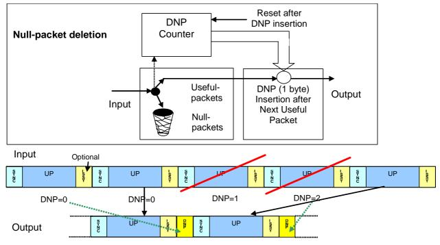
Figure 3: Null packet deletion scheme
