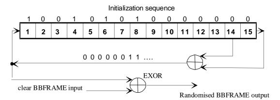
Figure 11: Possible implementation of the PRBS encoder
