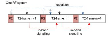
Figure 38: L1 signalling for a single RF system
