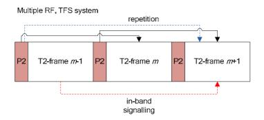
Figure E.5: L1 signalling for a TFS system
