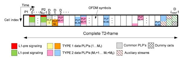
Figure 39: Mapping of data PLPs into the data symbols
