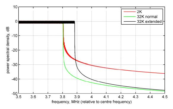
Figure 54(b): Detail of theoretical DVB-T2 spectrum for guard interval fraction 1/8 (for 8 MHz channels)
