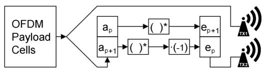
Figure 47: Multiple Input, Single Output, Encoder processing of OFDM payload cells
