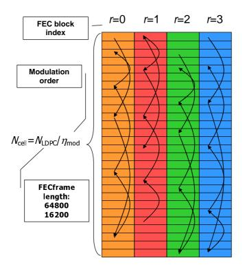
Figure 17: Cell Interleaving scheme
