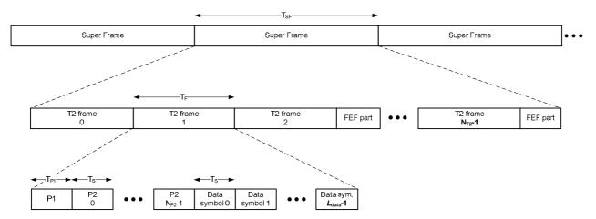
Figure 35: The DVB-T2 frame structure, showing the division into super-frames, T2-frames and OFDM symbols
