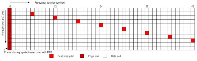
Figure K.8: Scattered pilot pattern PP8 (SISO)
