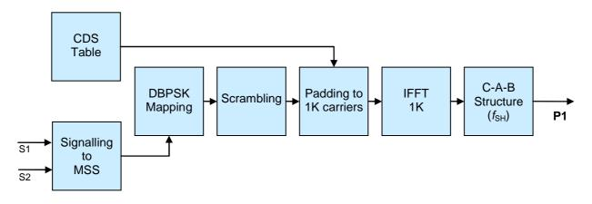
Figure 53: Block diagram of the P1 symbol generation
