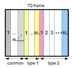
Figure 42: Allocation of  $M_{\text{common}}$  common PLPs,  $M_1$  data PLPs of type1 and  $M_2$  data PLPs of type 2 transmitted in one T2-frame
