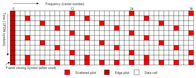
Figure K.1: Scattered pilot pattern PP1 (SISO)
