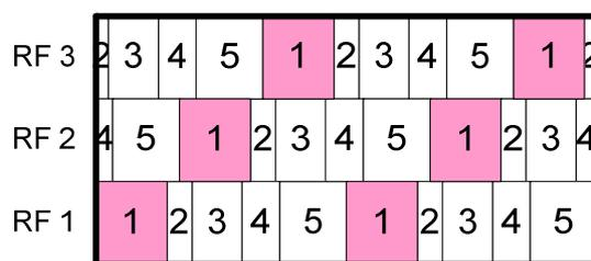
Figure E.9: Cell allocations for the sub-slices after folding
