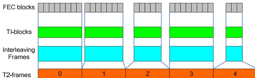
Figure 18(a): Time interleaving for  $P_1=1, I_{JUMP}=1, N_{TI}=1$
