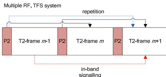
Figure E.6: L1 signalling for a TFS system
