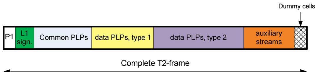
Figure 36: Structure of the T2-frame
