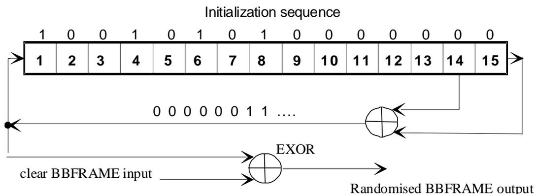
Figure 11: Possible implementation of the PRBS encoder
