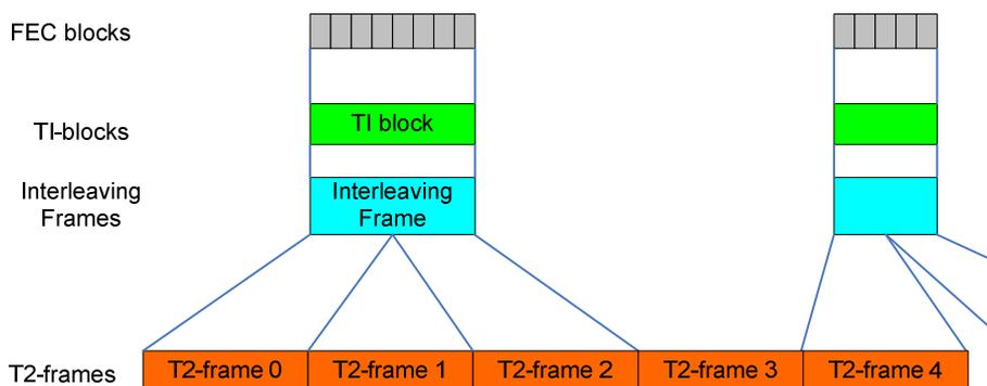
Figure 18(b): Time interleaving for  $P_1=2, I_{JUMP}=2, N_{TI}=1$
