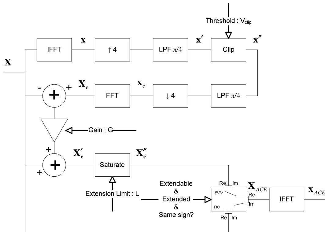
**Figure 48: Implementation of the Active Constellation Extension algorithm**
