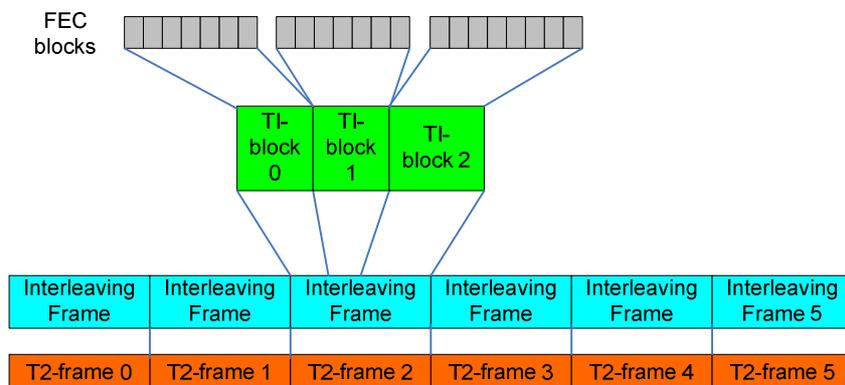
Figure 18(c): Time interleaving for  $P_1=1, I_{JUMP}=1, N_{TI}=3$
