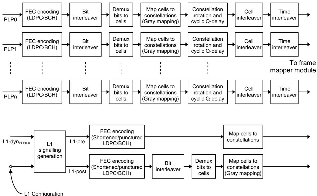
Figure 2(d): Bit Interleaved Coding and Modulation (BICM)
