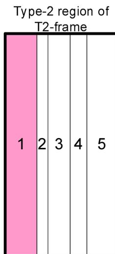
**Figure E.7: Capacity allocation of five type 2 data PLPs to one T2-frame**
