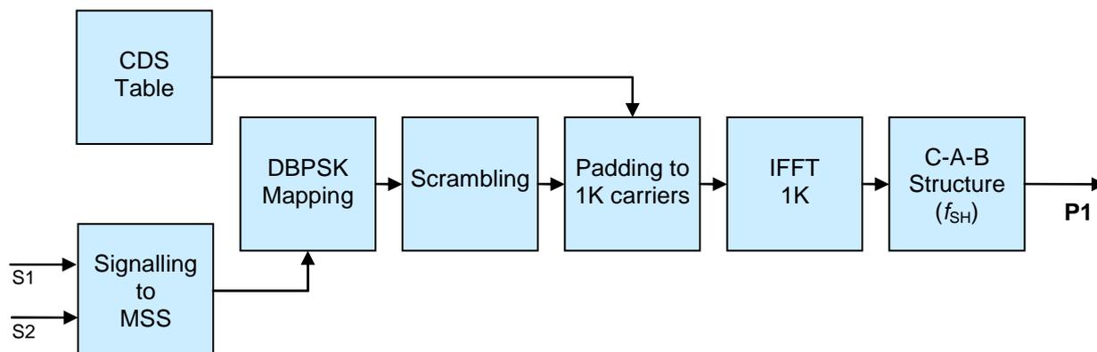
Figure 51: Block diagram of the P1 symbol generation
