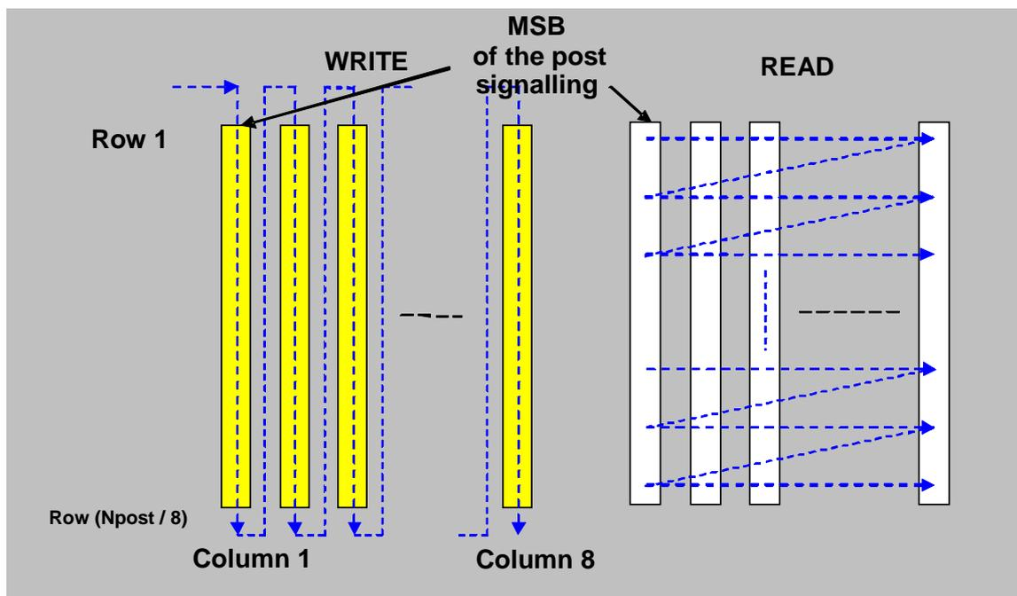
Figure 33: Bit Interleaving scheme for L1-post (16-QAM)
