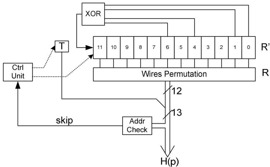
Figure 44(d): Frequency interleaver address generation scheme for the 8k mode
