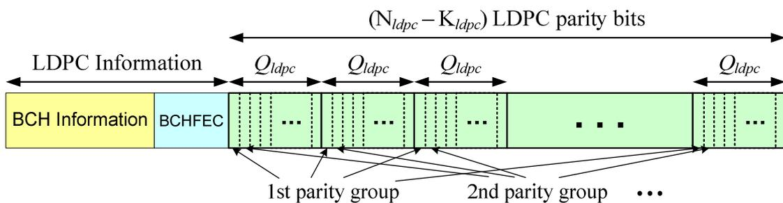
Figure 32: Parity bit groups in an FEC block
