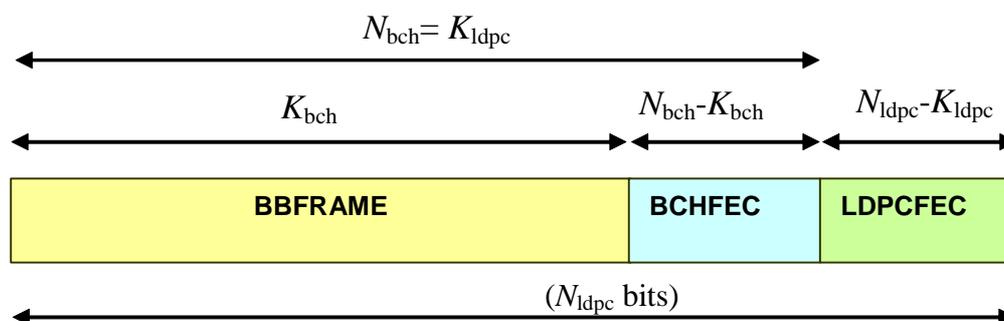
Figure 12: format of data before bit interleaving
