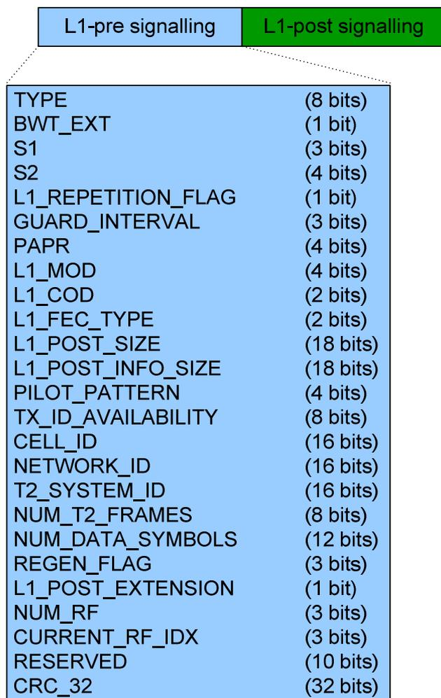
**Figure 25: The signalling fields of L1-pre signalling**
