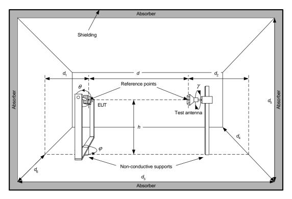
Figure 2: Typical anechoic chamber
