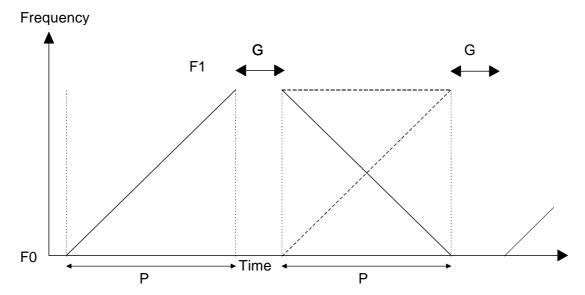
Figure F.2: Typical FMCW modulation scheme
