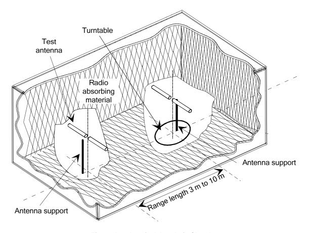
Figure A.1: A typical Anechoic Chamber
