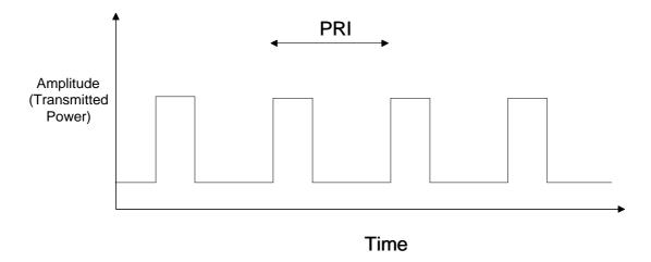
Figure F.1: Typical pulse modulation scheme
