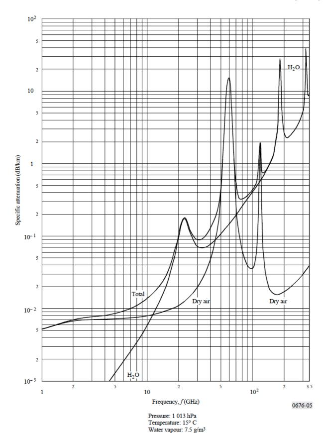
Figure G.1: Specific attenuation due to atmospheric gases in the band 1 GH to 350 GHz in dB/km
