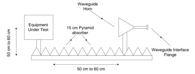
Figure 2: Example of the test fixture
