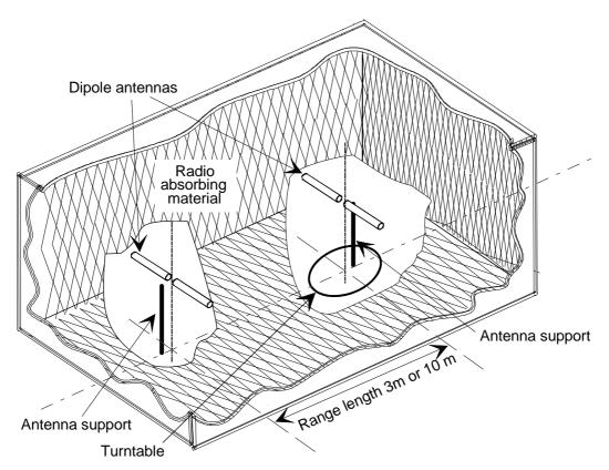
Figure 5: A typical Anechoic Chamber
