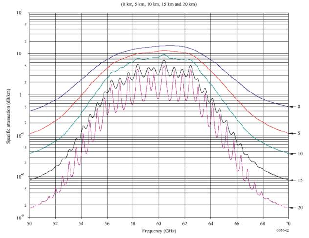
Figure C.2: Specific Atmospheric attenuation in the band 50 GHz to 70 GHz for different altitudes (0 km, 5 km, 10 km, 15 km and 20 km) [i.10]
