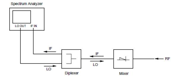
Figure 1: Set-up of measurement receiver, diplexer and mixer
