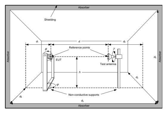
Figure 6: Typical anechoic chamber
