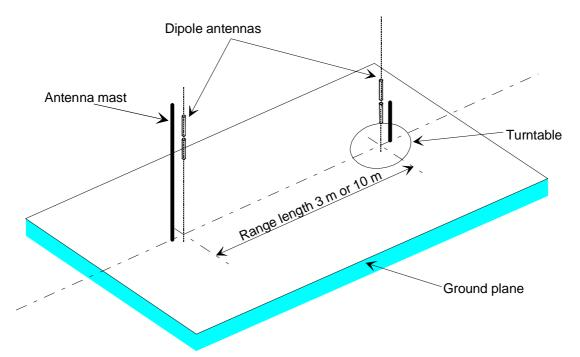
Figure 3: A typical Open Area Test Site
