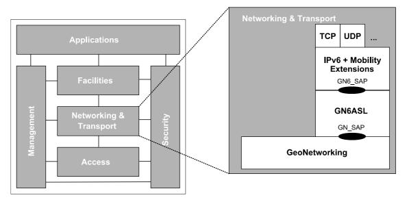
Figure 1: GN6ASL in the ITS station architecture
