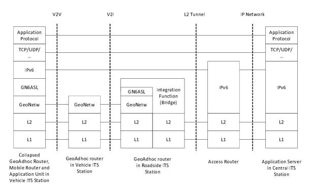
Figure 3: Separation of GeoAdhoc router and access router functions in a roadside ITS station
