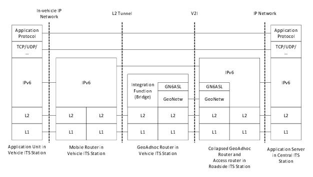
Figure 4: Separation of GeoAdhoc router and mobile router functions in a vehicle ITS station
