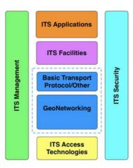
Figure 14: GeoNetworking protocol stack in an ITS station
