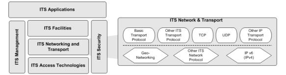
Figure 13: Details of the ITS networking and transport layer
