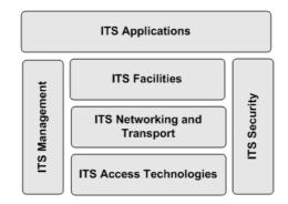
Figure 12: Reference protocol stack of an ITS station
