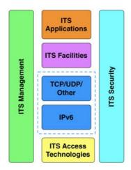
Figure 15: IPv6 stack in an ITS station
