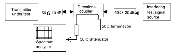
Figure 2: Measurement arrangement
