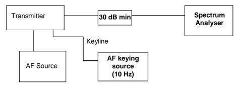
Figure 3: Measurement arrangement
