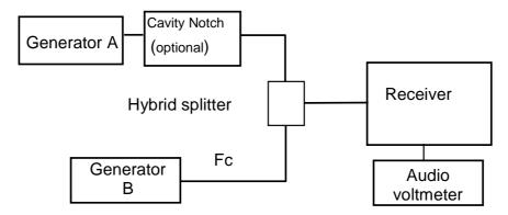
Figure 4: Measurement arrangement
