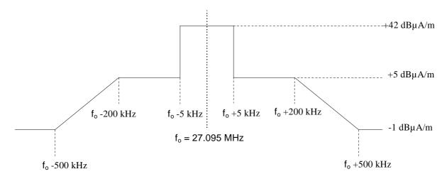
Figure 1: OBE transmitter mask
