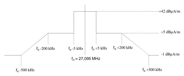
Figure 1: OBE transmitter mask
