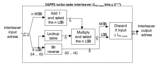
Figure 5.8: Turbo interleaver output address calculation procedure
