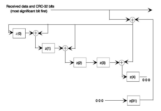
Figure A.1: 32 bits CRC decoder model
