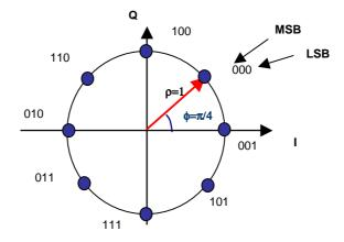
Figure 5.18: Bit mapping into 8PSK constellation
