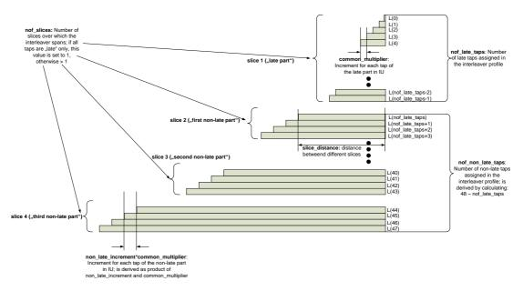
Figure 5.10: Interleaver branch delay description from receivers' point of view
