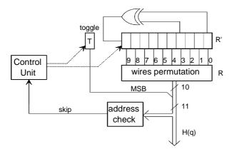
Figure 5.28: Symbol interleaver address generation scheme for the 2K mode
