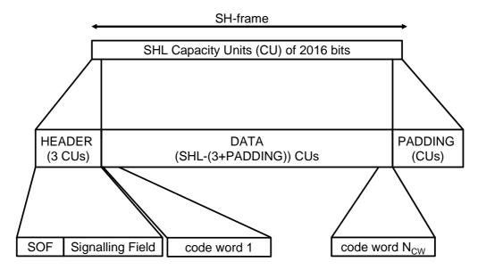
Figure 5.16: SH frame structure for TDM
