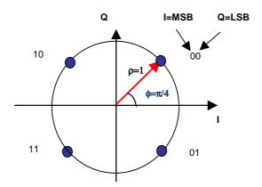
Figure 5.17: Bit mapping into QPSK constellation
