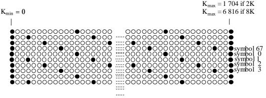
TPS pilots and continual pilots between  $K_{\text{min}} \text{and } K_{\text{max}}$  are not indicated
