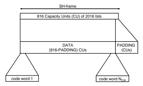
Figure 5.15: SH frame structure for OFDM
