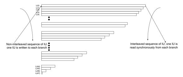
Figure 5.9: Conceptual diagram of the time interleaver
