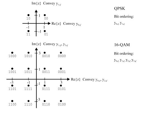
Figure 5.31: The QPSK, 16-QAM mappings and the corresponding bit patterns (non-hierarchical, and hierarchical with  $\alpha$  = 1)
