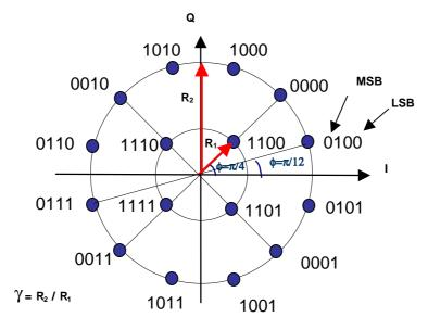
Figure 5.19: Bit mapping into 16APSK signal constellation
