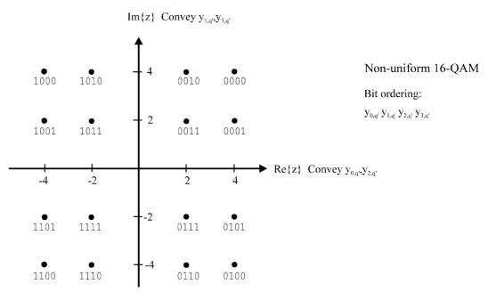
Figure 5.32: Non-uniform 16-QAM mappings with  $\alpha = 2$
