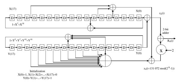
Figure 5.25: Configuration of PL scrambling code generator
