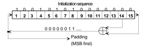
Figure 5.13: Implementation of the padding part generator for SH frame completion
