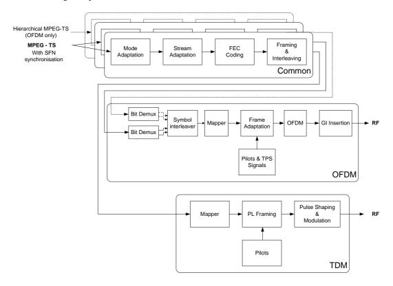
Figure 4.1: Functional block diagram of the DVB-SH transmitter (Either TDM or OFDM configurations)
