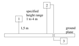
NOTE: 1: Device under test. 2: Test antenna.
