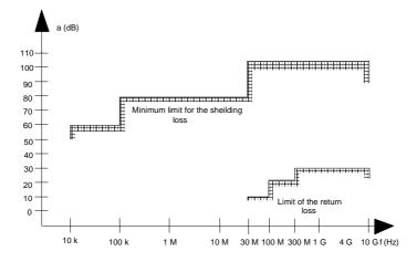
Figure B.2: Specification for shielding and reflections
