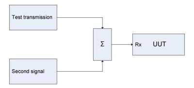
Figure 3: A possible conducted measurement arrangement
