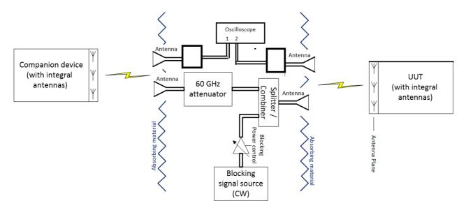
Figure 2: Test Set-up for verifying the adjacent channel rejection of an equipment
