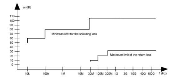
Figure C.2: Specification for shielding and reflections
