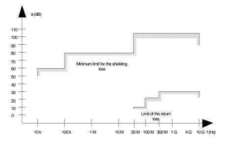
Figure C.2: Specification for shielding and reflections
