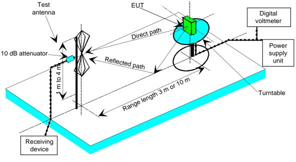
Typical measuring arrangement common for ground plane test sites is presented in the figure B.4.
