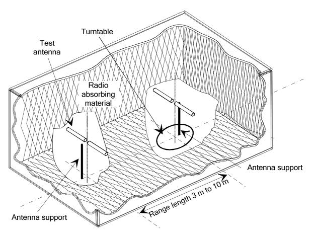
Figure B.1: A typical anechoic chamber
