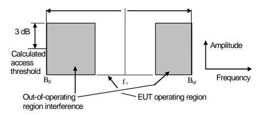
Figure 2: Spectrum mask for test of clause 5.3.8.1.1.1
