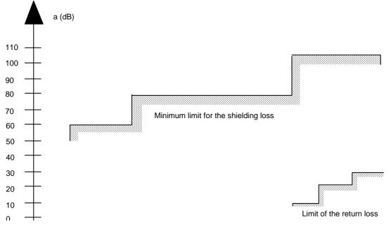
Figure B.4: Specification for shielding and reflections
