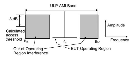
Figure 3: Spectrum mask for test of clause 5.3.8.1.2.1
