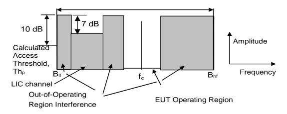
Figure 4: Spectrum mask for test of clause 5.3.8.1.4.1
