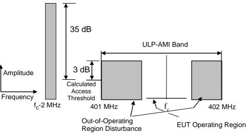
Figure 1b: Spectrum Mask for Test (f<sub>c</sub> - 2 MHz) of clause 5.3.7.1
