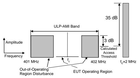
Figure 1a: Spectrum Mask for Test (f<sub>c</sub> + 2 MHz) of clause 5.3.7.1
