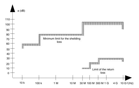
Figure B.2: Specification for shielding and reflections
