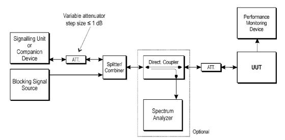
Figure 9: Test Set-up for receiver blocking
