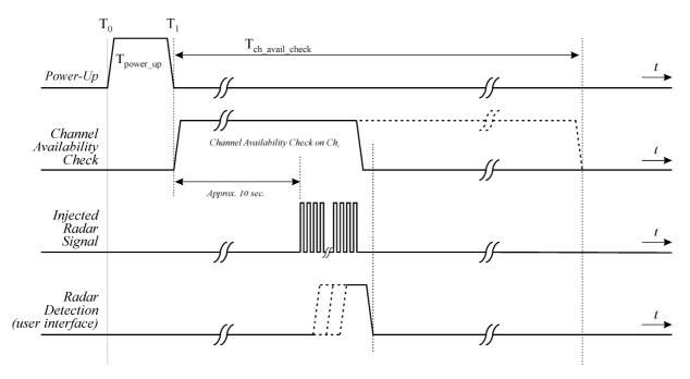
Figure 6: Example of timing for radar testing during the Channel Availability Check
