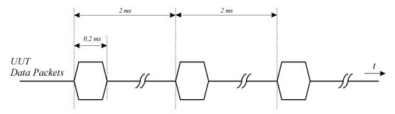
Figure 2: An example of the test transmission sequences
