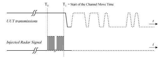
Figure 7: Example of timing for radar testing during In-Service Monitoring
