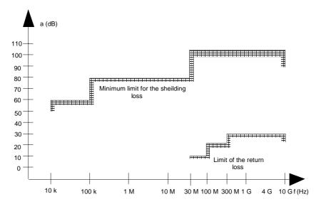
Figure B.2: Specification for shielding and reflections
