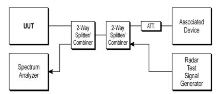
NOTE: UUT can be any type of FWA Device under test. An Associated Device is the equipment required for the UUT to establish a communication link.
