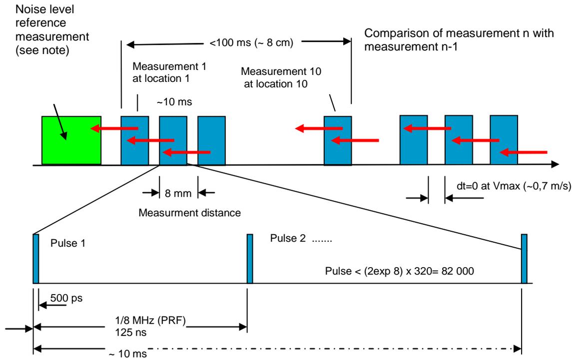
NOTE: Internal equipment noise measurement is done without antenna. In a second step the antenna will be switched on and an additional noise measurement will be done which is compared to the measurement without antenna. No transmitting included so far. Hereafter the intrinsic material measurement will be done transmitting included.
