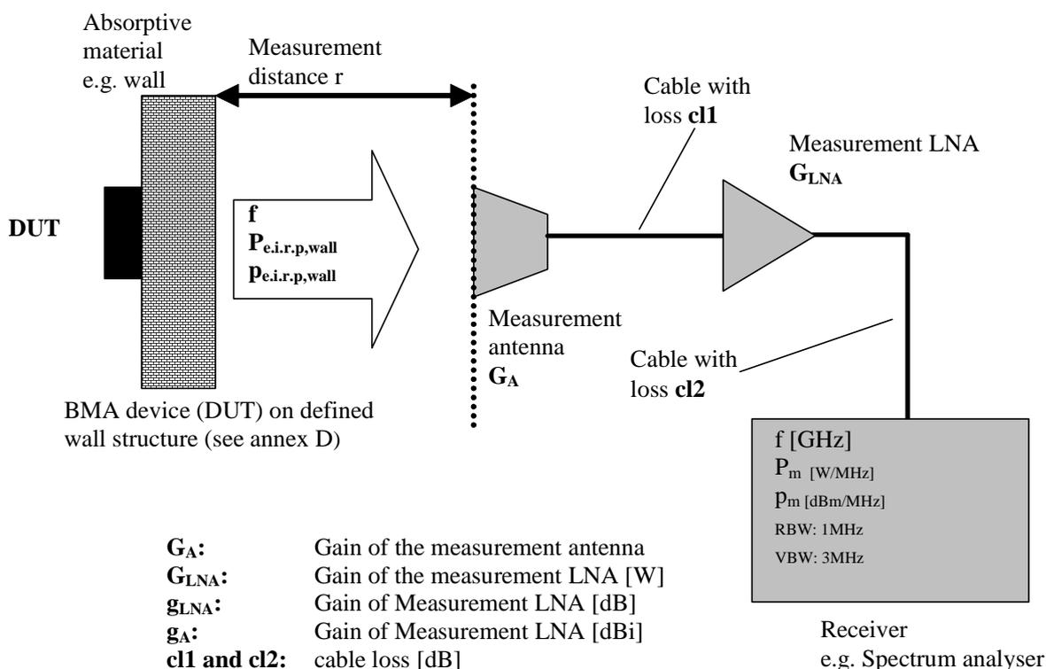
**Figure 3: Test set-up for e.i.r.p measurement**
