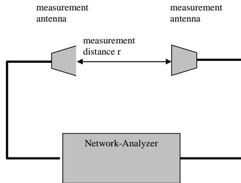
**Figure D.1: Calibration setup**
