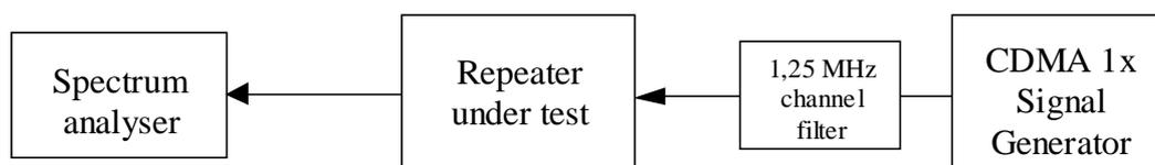
Figure E.1: Measuring system set-up for conducted unwanted emission
