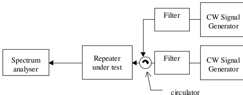
Figure E.3: Measuring system set-up for input intermodulation
