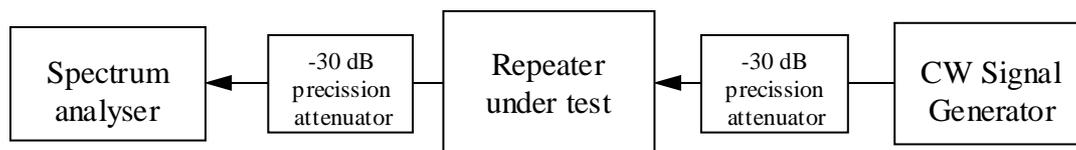
Figure E.4: Measuring system set-up for out of band gain
