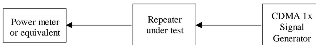
Figure E.2: Measuring system set-up for maximum output power
