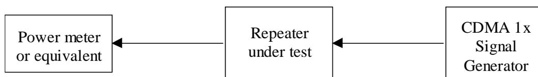
Figure E.5: Measuring system set-up for Adjacent Channel Rejection Ratio
