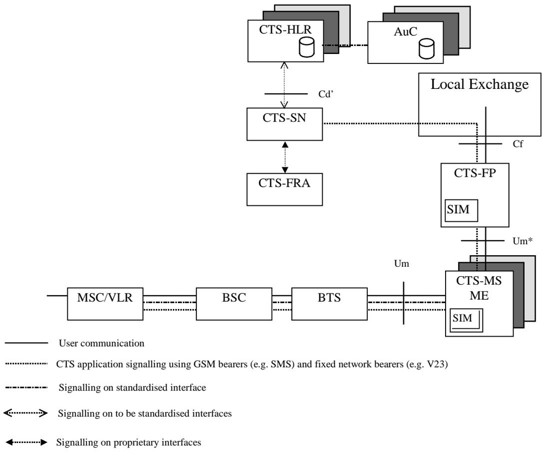
**Figure 6: Simplified CTS reference model (limited enrolment control)**
