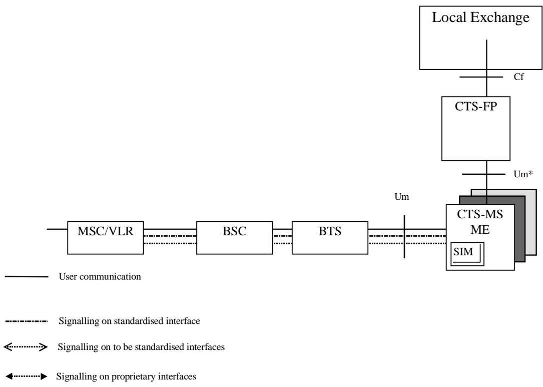
When the CTS-FP is used in licence exempt mode, the CTS-FP owner does not need to have a subscription with a CTS operator. Therefore the CTS-FP can work without CTS-SIM card and no exchange with a CTS-SN is necessary.
