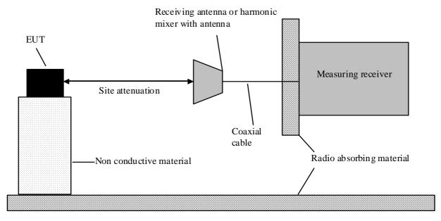
Figure A.5: Example of a test site above 18 GHz with one reflecting surface
