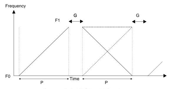
Figure G.2: Typical FMCW modulation scheme
