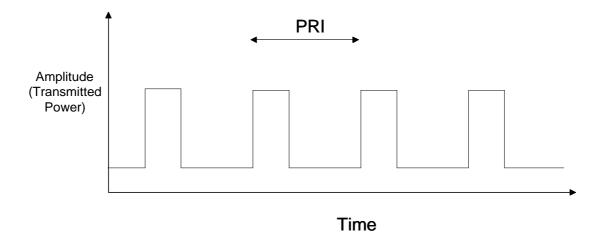
Figure G.1: Typical pulse modulation scheme
