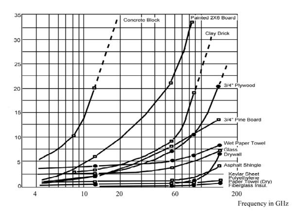
Figure H.3: Material Absorption at High Frequency in the frequency range from 3 GHz to 200 GHz in dB
