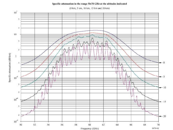
Figure H.2: Specific Atmospheric attenuation in the band 50 GHz to 70 GHz for different altitudes (0 km, 5 km, 10 km, 15 km and 20 km) [i.6]
