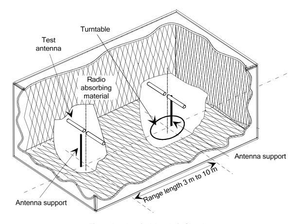
Figure A.1: A typical Anechoic Chamber
