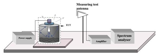
Figure 3: An example of test set-up for emission measurement
