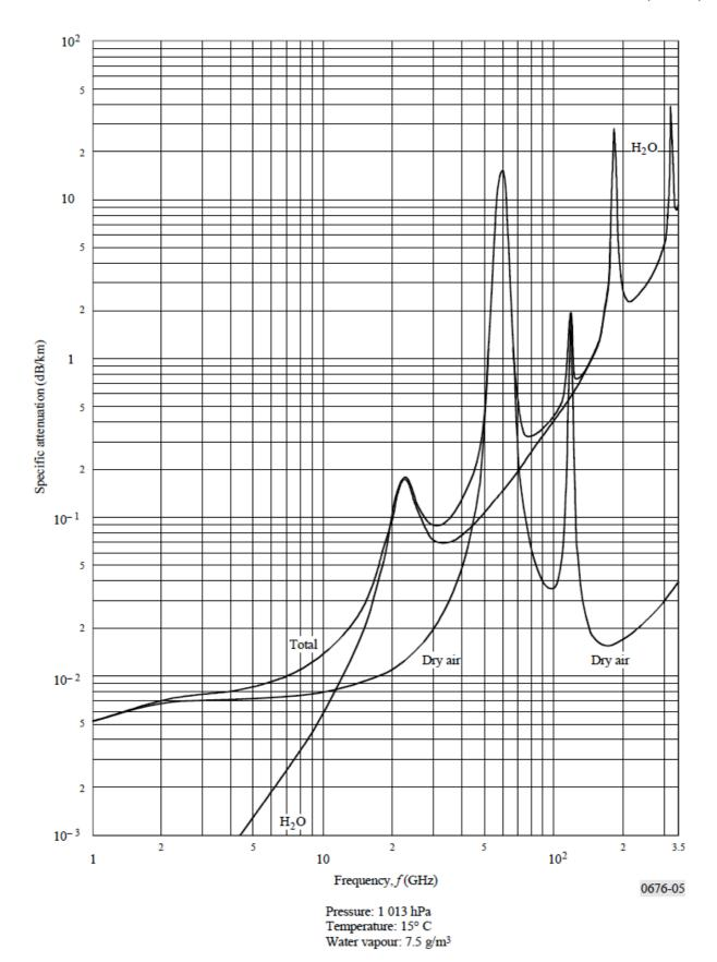
Figure H.1: Specific attenuation due to atmospheric gases in the band 1 GHz to 350 GHz in dB/km
