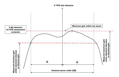
Figure 2: Gain ripple for a sectored antenna
