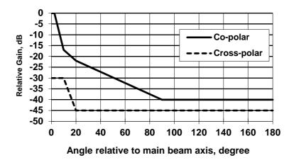
Figure 7: Class DN4 terminal station antenna
