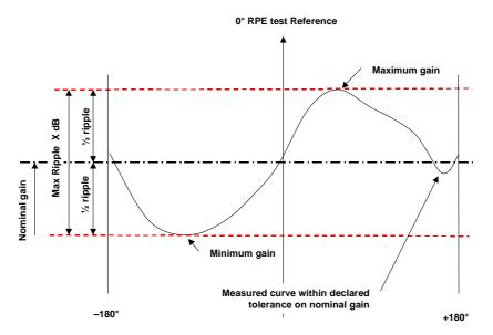
NOTE: Figure 1 shows the relationship between the X dB gain ripple, measured minimum and *maximum gains* in the *azimuth plane*, and the declared *nominal gain* and *gain tolerance* of an omnidirectional antenna.
