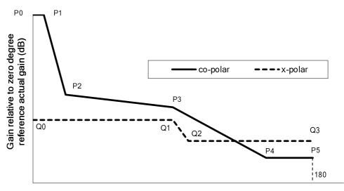
Angle relative to zero degree reference (deg)
