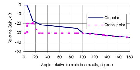
Figure 4: Class DN1 terminal station antenna
