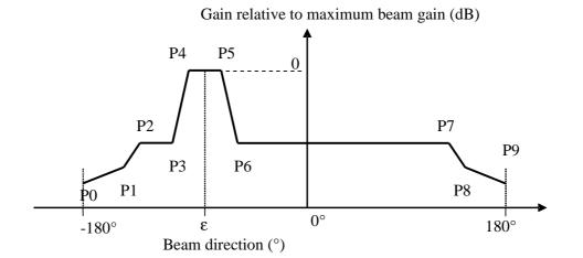
Figure 8: Azimuth RPEs for linear polarized multi-beam sector antennas 3 GHz to 5,9 GHz (defined for each beam)
