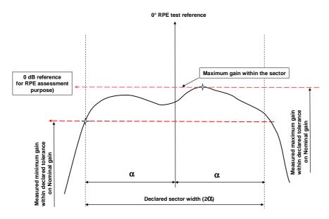
Figure 3: Gain ripple for a sectored antenna
