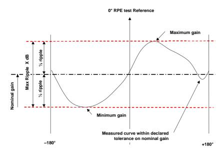
NOTE: Figure 2 shows the relationship between the X dB gain ripple, measured minimum and maximum gains in the azimuth plane, and the declared nominal gain and tolerance of an omnidirectional antenna.
