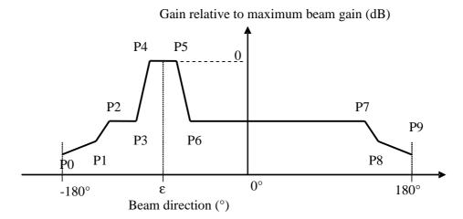
Figure 5: Azimuth RPEs for linear polarized multi-beam sector antennas 3 GHz to 5,9 GHz (defined for each beam)
