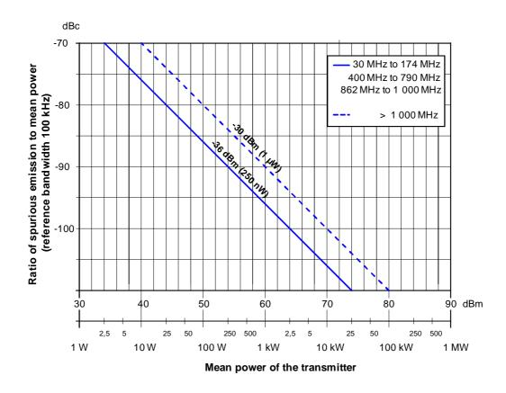
Figure 4.1: Spurious emission limits for DVB-T transmitters (100 kHz reference bandwidth)
