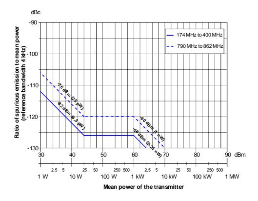
Figure 4.2: Spurious emission limits for DVB-T transmitters (4 kHz reference bandwidth)
