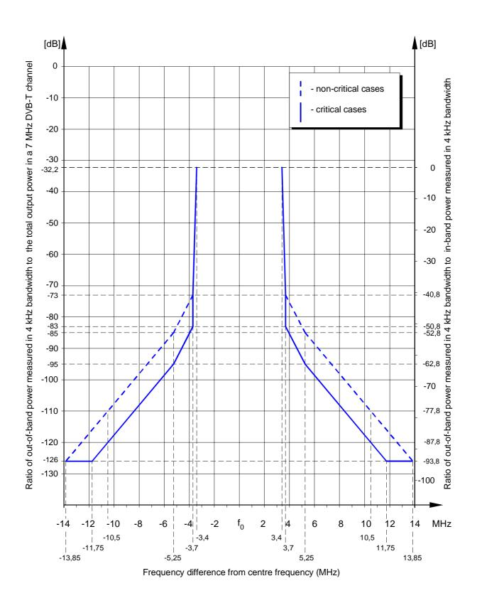
Figure 4.3: Out-of-band limits for DVB-T transmitters ≥ 25 W in 7 MHz channels
