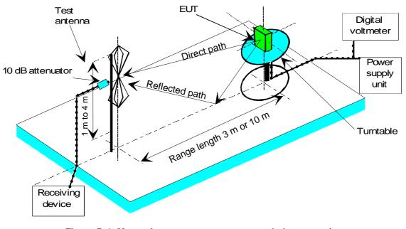
Figure B.4: Measuring arrangement on ground plane test site (OATS set-up for spurious emission testing)
