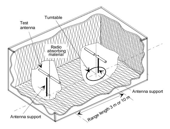
Figure B.1: A typical anechoic chamber
