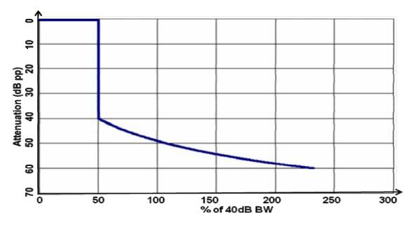
The maximum radiated Out Of Band-emission power level shall not exceed the limits given in figure 1.
