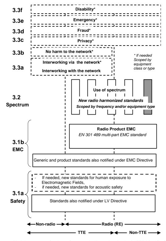
Figure 1: Modular structure for the various standards used under the R&TTE Directive [2]
