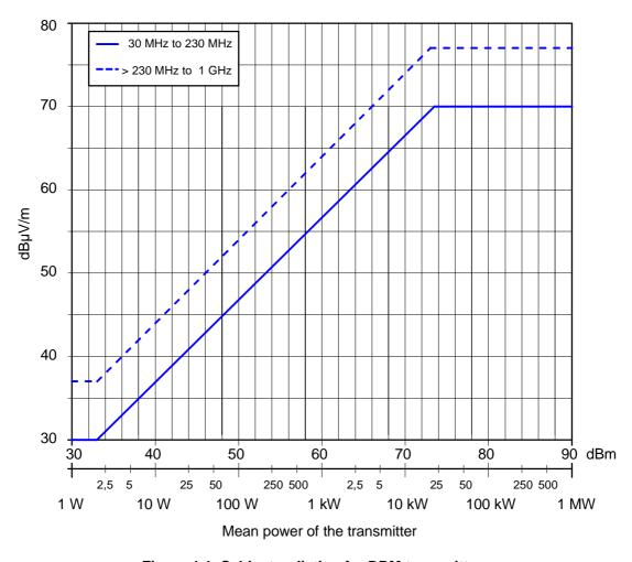
Figure 4.4: Cabinet radiation for DRM transmitters
