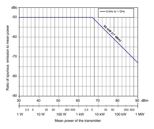
Figure 4.1: Spurious emission limits for DRM transmitters
