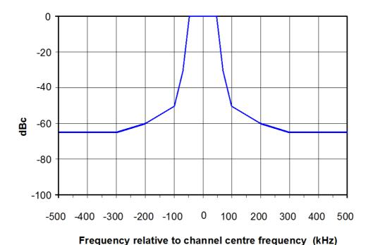
Figure 5: Out-of-band emission limits for DRM transmitters operating between 30 MHz and 300 MHz
