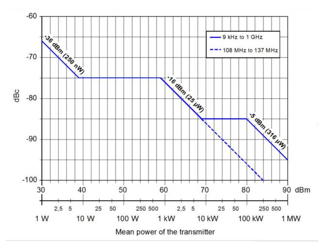
Figure 2: Spurious emission limits for DRM transmitters operating between 30 MHz and 300 MHz
