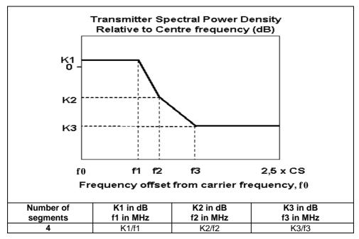
Figure 3: Four segment spectrum mask
