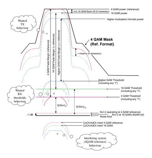
Figure I.2: Example of nodal co-channel interference (reference modulation format 4QAM):
