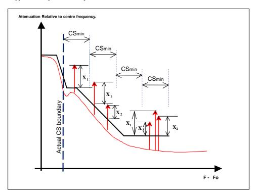
Figure 7: CW lines exceeding the spectrum mask (typical example)
