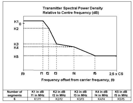
Figure 5: Six segment spectrum mask
