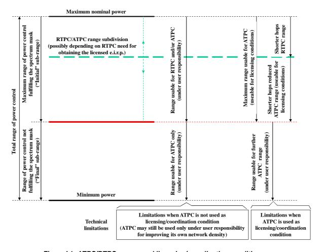
Figure I.1: ATPC/RTPC ranges and licensing/coordination conditions
