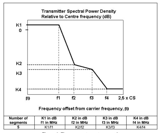
Figure 4: Five segment spectrum mask
