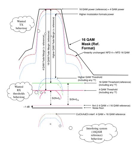
Figure I.3: Example of nodal co-channel interference (reference modulation format 16QAM):
