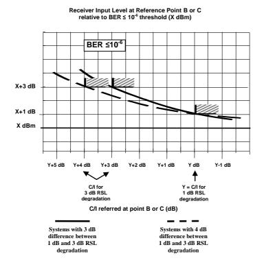
Figure J.1: Interference threshold degradation versus C/I (typical behaviour)
