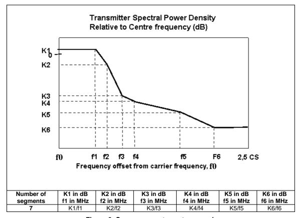
Figure 6: Seven segment spectrum mask
