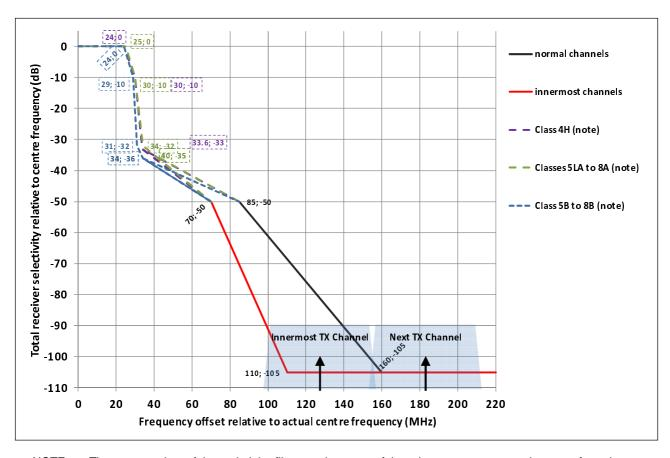
NOTE: The corner points of the main lobe filter are the same of the relevant spectrum masks a part from the +2 dB (K1 value) brought down to 0 dB; see ETSI EN 302 217-2 [18].
