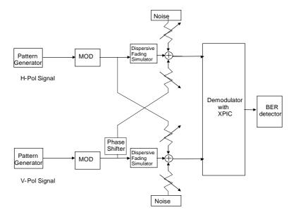
Figure D.1: IF measurement test set
