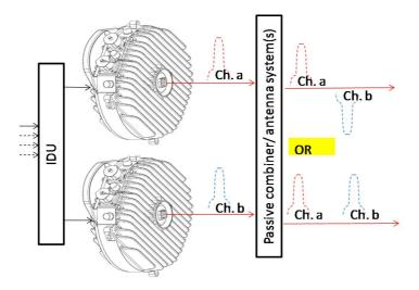
Figure C.1: Examples of Multi-channel system
