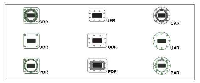
Figure 2: Waveguide Flange Shapes
