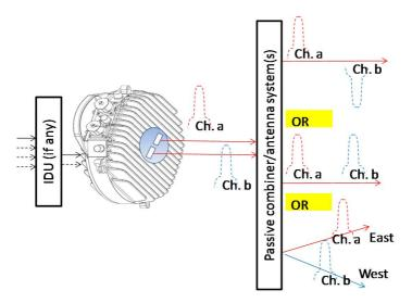
Figure C.3: Example of Channels aggregation/dual-port equipment
