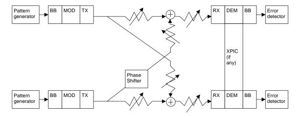
Figure D.2: RF measurement test set
