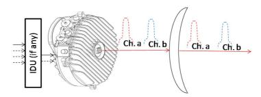
Figure C.2: Example of channels aggregation/single-port equipment
